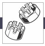
Slotted nuts have slots that extend all the way through the nut, while castle nuts have slots that are only cut into the upper portion of the nut. This leaves a solid "turret" at the base of the nut.
