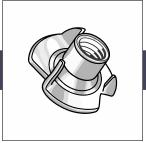
T-nuts often have hooks or serrations on the prongs that dig into a wooden work piece as the bolt is tightened from the opposite side of the piece, providing better retention.
