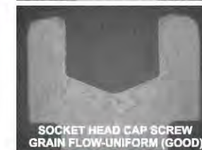
SOCKET HEAD CAP SCREW GRAIN FLOW-UNIFORM (GOOD)
