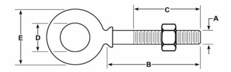
Forged carbon steel, heat treated, hot galvanized. Heavy hex nut according to ASME/ANSI B18.2.2.
